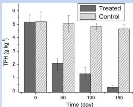
Reductions in TPH concentrations during bioremediation (bar is  $\pm$  standard deviation for five measurements).
