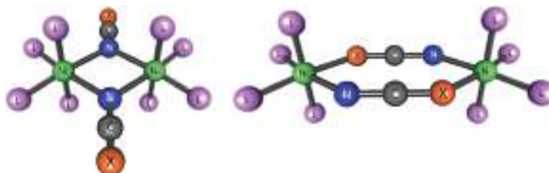
Fig. 1. Possible double bridging modes of cyanato and thiocyanato ions in binuclear nickel(II) complexes; “end-on” on the left and “end-to-end” mode on the right; X= O or S; L – spectator ligands.
