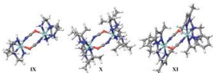
Fig. 3. “End-to-end” cyanato double bridged Ni(II) binuclear complexes.
