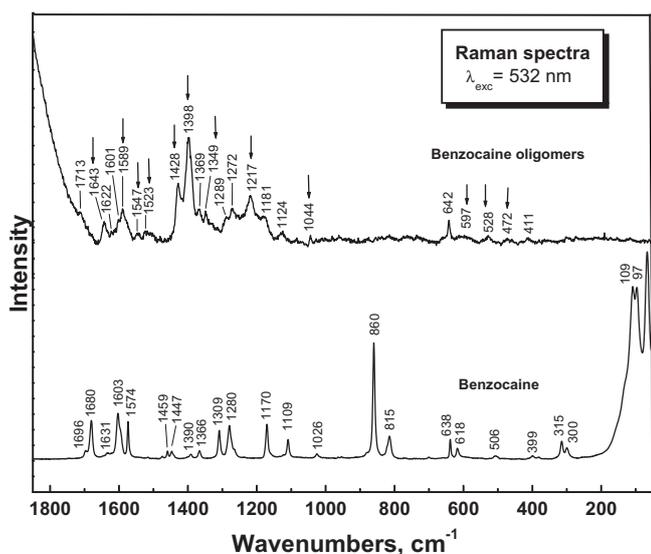
**Fig. 5.** Raman spectra of benzocaine and its oligomers in the wavenumber region 1850–50  $\text{cm}^{-1}$ ; excitation wavelength 532 nm. The new bands which appeared in the spectrum of oligomers in comparison with the spectrum of monomer are marked with an arrow.
