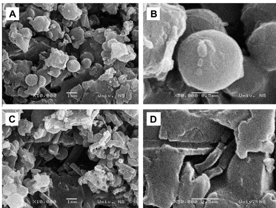
Fig. 2. Scanning electron micrographs of oligobenzocaines (A, C, and D different parts of the same sample in two magnifications; B is magnified part of A).
