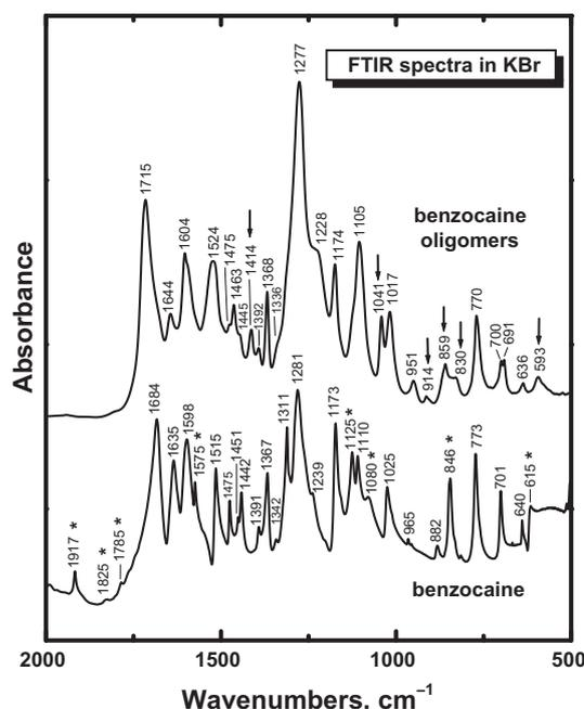
Fig. 4. FTIR spectra of benzocaine and its oligomers in the wavenumber region 2000–500 cm<sup>-1</sup>. The new bands which appeared in the spectrum of oligomers in comparison with the spectrum of monomer are marked with an arrow; the bands of monomer which disappeared in the spectrum of oligomers are marked with an asterisk.
