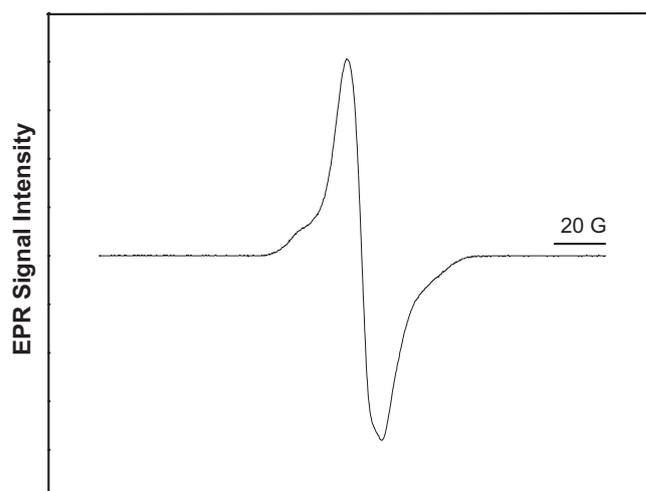
**Fig. 6.** EPR spectrum of benzocaine oligomers.
