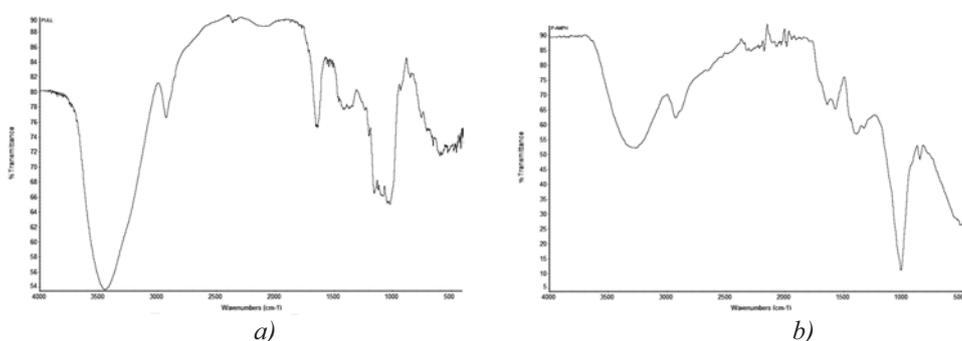
**Fig.2:** FT-IR spectra of pullulan (a) and pullulan-amphotericin B conjugates (b)
